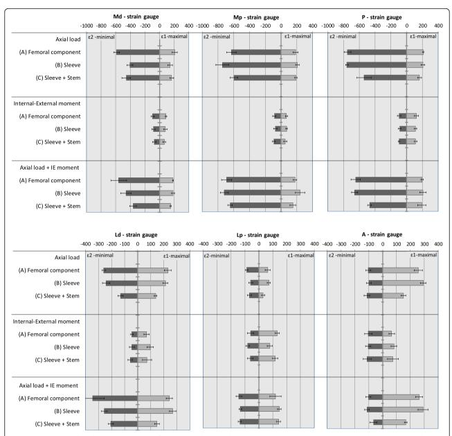
**Fig. 4** Mean and standard deviation (error bars) of the measured principal strains ( $\epsilon$ 1 - maximal and  $\epsilon$ 2 - minimal) at each strain gauge Md (medial distal), Mp (medial proximal), P (posterior), A (anterior), Ld (lateral distal) and Lp (lateral proximal) for each construct technique and load case
