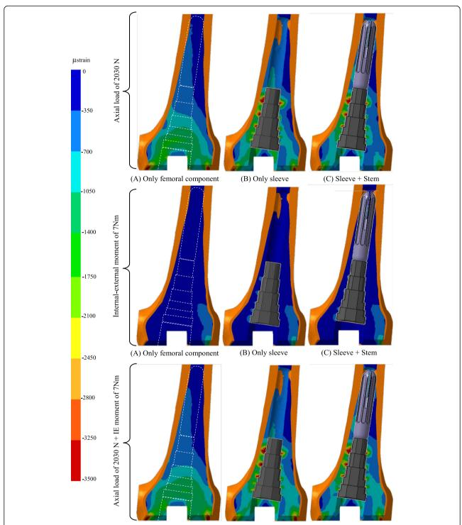
**Fig. 5** Minimal principal strains in cancellous bone for the axial load case (upper row), internal-external moment load case (middle row) and axial load + internal-external moment load case (lower row) on the construct technique only with femoral component (left column), with sleeve (centre column) and with sleeve and stem (right column). The colour gradient specifies the range of principal strains
