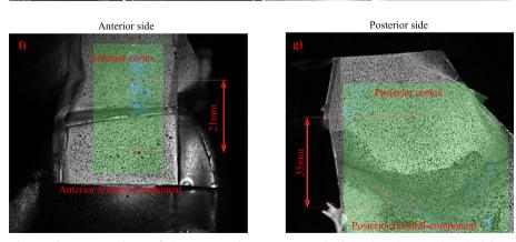
Fig. 2 a Loading machine and experimental setup; b Strain gauges locations at Lateral side Lp (lateral proximal) and Ld (lateral distal); c Strain gauge location at Anterior side (A); d Strain gauges locations at Medial side Mp (medial proximal) and Md (medial distal); e Strain gauge location at Posterior side (P); f DIC image - stochastic pattern at Anterior femur side; g) DIC image - stochastic pattern at Posterior femur side
