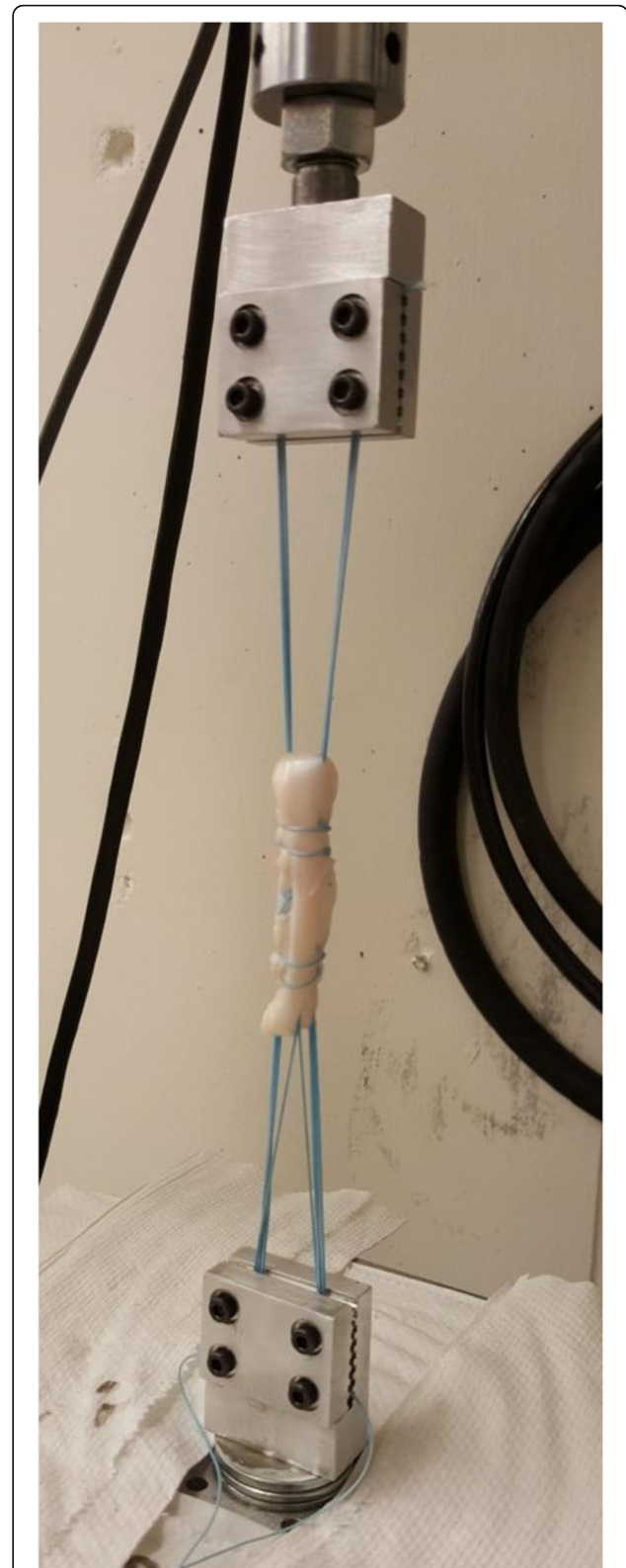
Fig. 2 A quadrupled tendon suspended using No. 5 suture from clamps in the MTS machine
