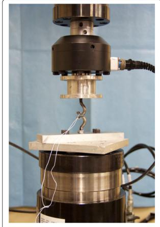
**Fig. 1** Testing Apparatus. MTS Bionix Servohydraulic Test Frame with suture located between two eyelets
