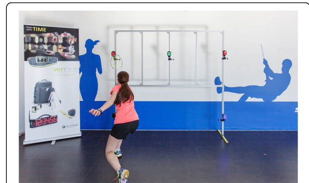
Fig. 3 A badminton player practicing reaction task using the Microgate Witty SEM system (Microgate, Bolzano, Italy). The Microgate Witty SEM shown here consist of a framework holding three LED lights that illuminate green in a random order. In this set-up, the player has to respond quickly and move the racquet in front of the LED that turns green
