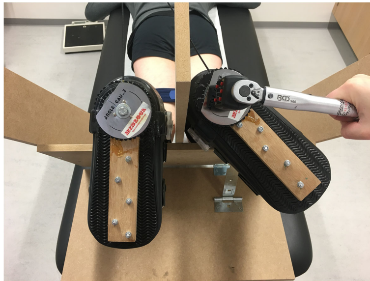
Fig. 1 External rotation with 6 Nm torque
