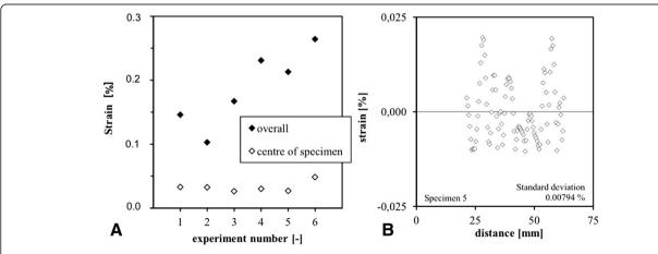
**Figure 5** Overview of the obtained scatter in all specimens both at the centre part and the whole tendon (A). A typical example of central area for specimen 5 is shown in detail (B).
