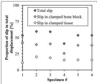
**Figure 6** The difference between DIC 1 and DIC 2 measurements was plotted for each specimen. In this way, the slip in the grips was quantified. A distinction between the bone block clamp and the tissue clamp was made with the latter showing significant less slip.
