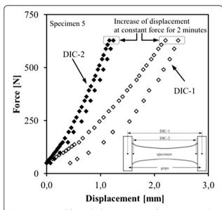
**Figure 3 A typical force-displacement curve of specimen 5.** Both loading and unloading phase are shown. At maximum load, the specimens were kept at constant force for roughly two minutes before unloading. For the displacements measured on the specimens (DIC-2) the difference between loading and unloading was allocated to hysteresis. For the grip-to-grip measurements (DIC-1), the difference was mainly the consequence of slip in the grips.
