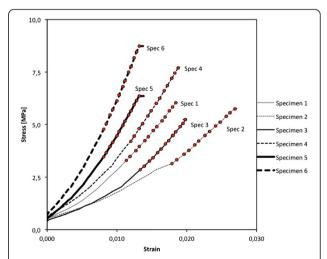
**Figure 4 Stress-strain curves for all 6 specimens.** The marks were placed on the linear part of the curve. The E modulus was determined from the slop of this part of the curve for each specimen. Specimen 1, 2 and 3 were not pre-loaded. Specimen 4, 5 and 6 were pre-loaded. Cfr Table 2.
