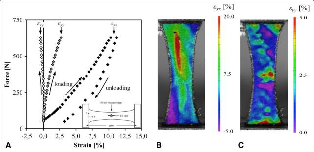
Figure 7 Evolution of strain components over central area of specimen 5 as function of the applied force (A). The shear strain  $\varepsilon_{xy}$  remained close to zero during the experiment. The corresponding strain maps at maximal load showing the transverse strains  $\varepsilon_{xx}$  (B) and longitudinal strains  $\varepsilon_{yy}$  (C) are also given.
