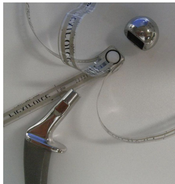
Fig. 1 A photograph of an instrumented prosthesis, which is reassembled, and a stem. Four pressure sensors are placed on the faces of a cube-shaped part
