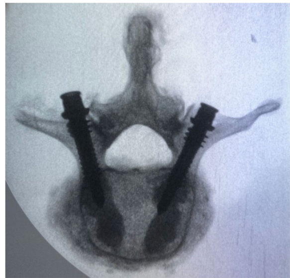
Fig. 4 Example of radiograph after surgical treatment and biomechanical testing, which shows pedicle integrity
