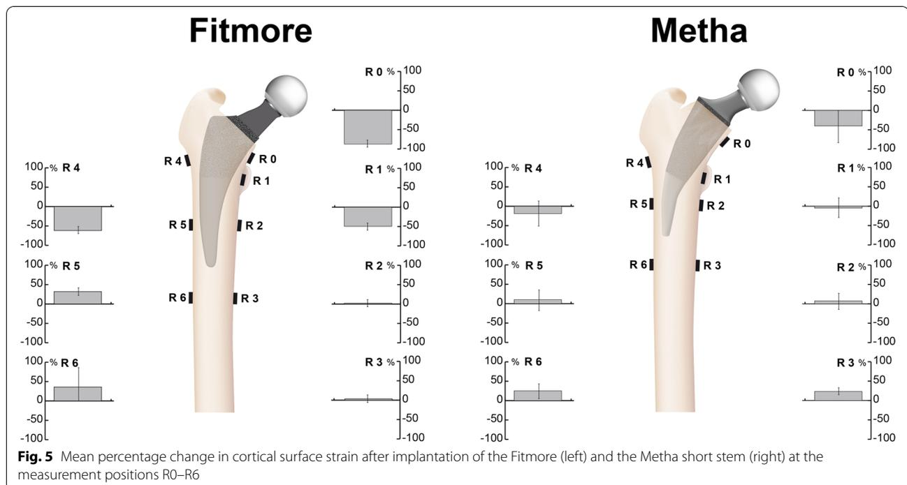
**Fig. 5** Mean percentage change in cortical surface strain after implantation of the Fitmore (left) and the Metha short stem (right) at the measurement positions R0–R6
