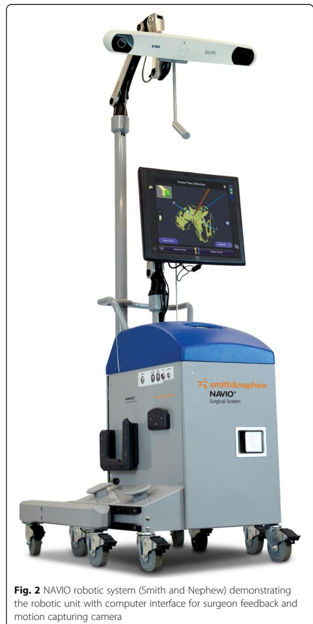
**Fig. 2** NAVIO robotic system (Smith and Nephew) demonstrating the robotic unit with computer interface for surgeon feedback and motion capturing camera
