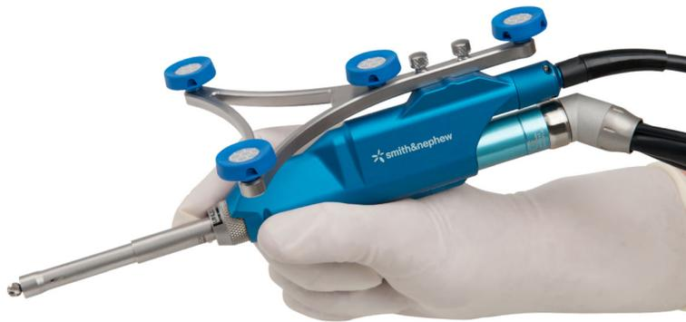
**Fig. 3** Cutting burr connected to the robotic unit in image 2. The handpiece delivers the surgical plan determined by the surgeon. Whilst the surgeon still has some control over the movement of the cutting tool, some robotic systems are designed to ‘cut-out’ when the instrument strays from planned surgical resection margins on the plan
