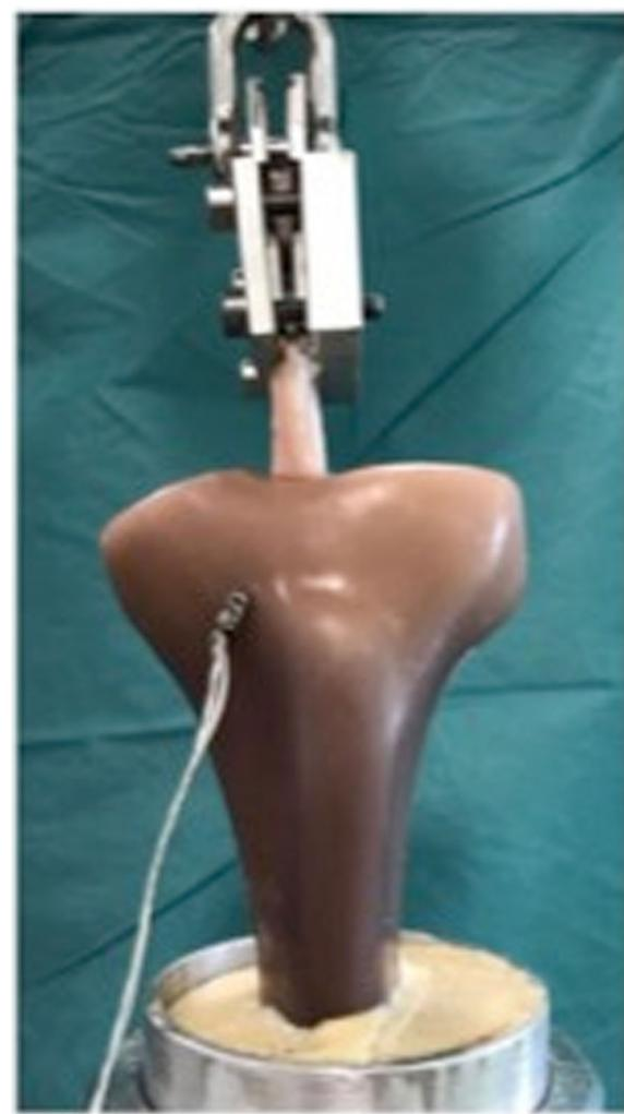
**Fig. 1** Extracortical tibial fixation devices were used in this study. Porcine tendons were mounted onto sawbone™ tibiae
